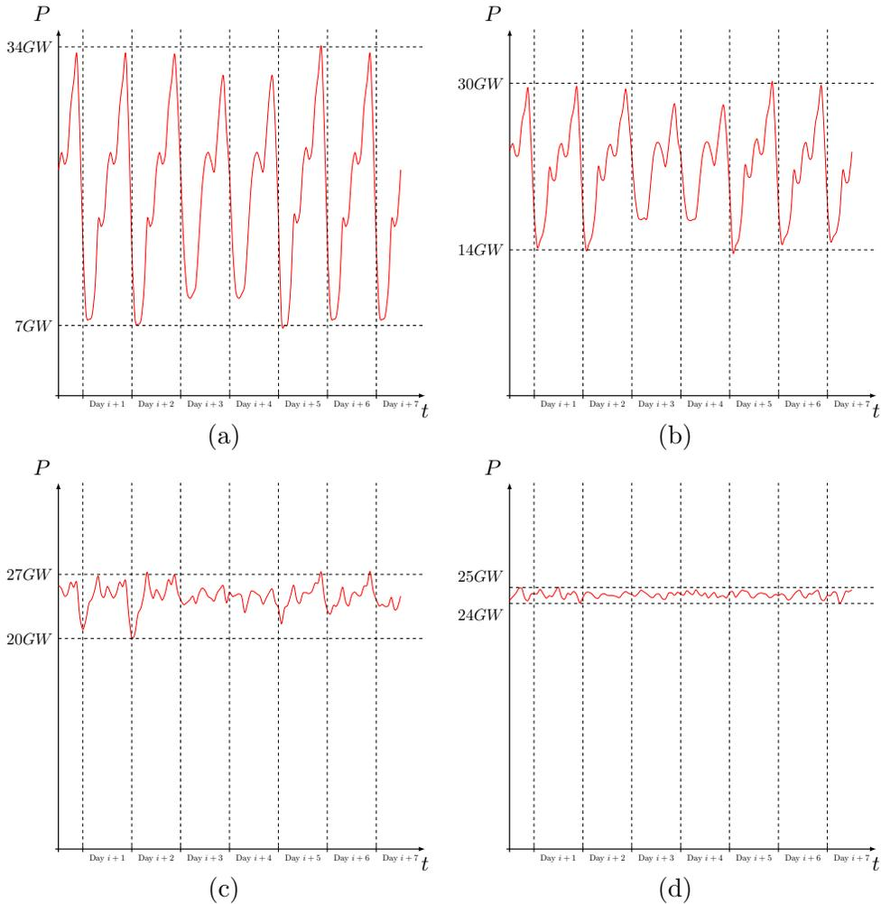
Figure 3: Operation example of the swarm intelligence algorithm for Smart Grid management: a) without controllable consumption, b) 25% of controllable power consumption, c) 50% of controllable power consumption and d) 100% of controllable power consumption.
