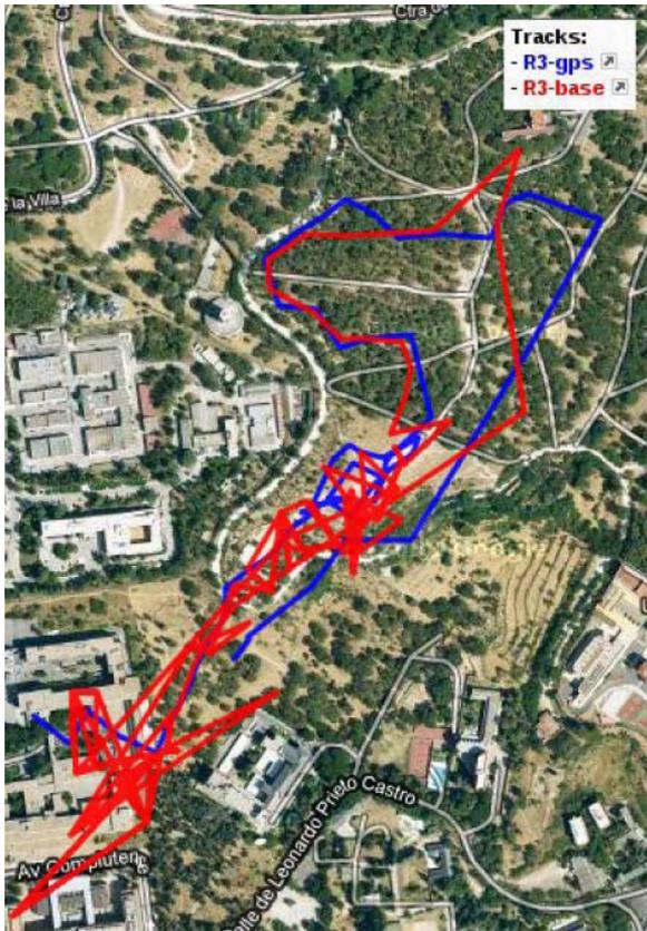
Fig. 6. Tracking results of a secondary node. (Blue in online version) Real trajectory as retrieved from the GPS module and (red in online version) trajectory reported by the base station.
