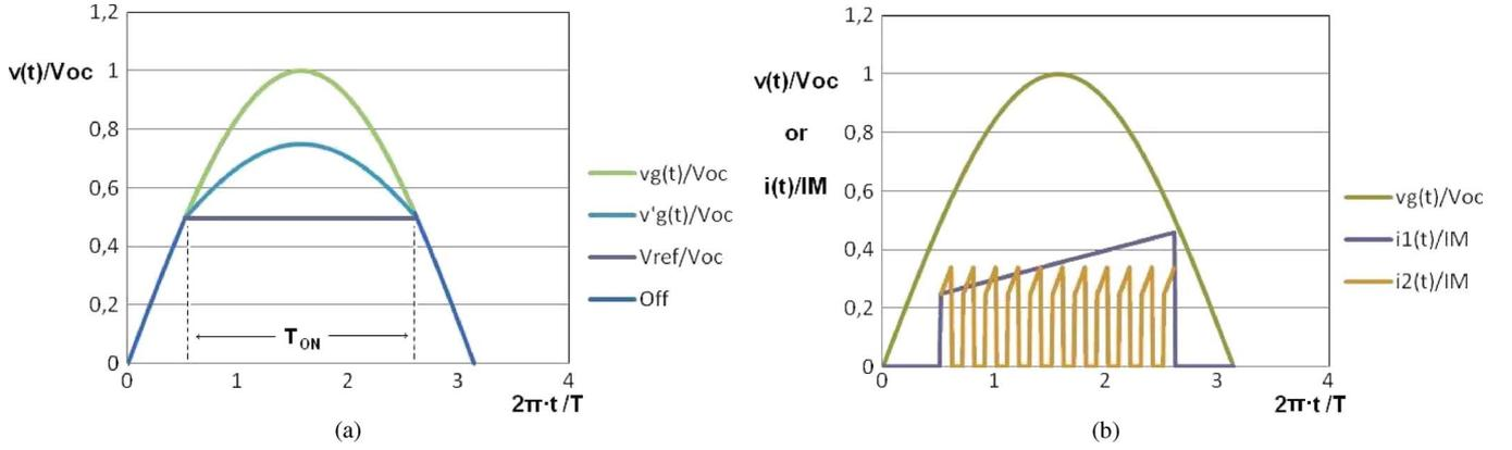
Fig. 2. Typical converter normalized input current waveform as a function of normalized time under different load conditions. (a)  $T_{ON}$  is the normalized time during which the converter is on per semicycle. (b) Normalized open-circuit generator voltage in a semicycle is given as a reference.
