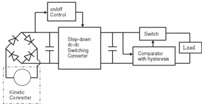
Fig. 1. Secondary node harvester block diagram.
