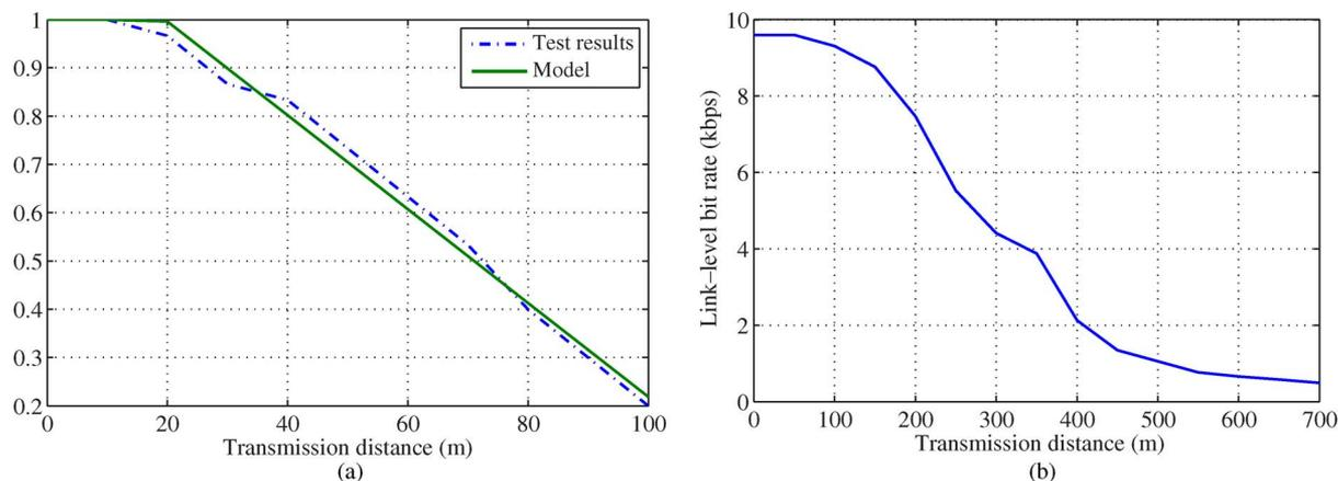
Fig. 3. Radio-link hardware tests. (a) Secondary-link probability of successful reception. (b) Repeater-link throughput.
